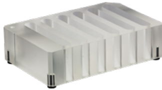
Figure 2 Column Holder D (note top left mark for correct orientation)
