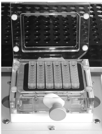
Figure 6 NucleoSpin® Plasmid Filter Strips inserted into Column Holder B placed in the manifold top on the BioRobot® 9600.
