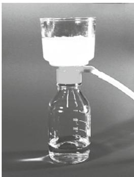
**Figure 2** Correct use of the NucleoBond® Bottle Top Filter
