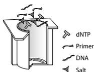
PCR products are loaded directly onto the **NucleoFast® 96 PCR** filter membrane.
