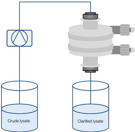
Unfiltered Crude lysate → 20 µm → 5 µm → 0.45 µm Clarified lysate
