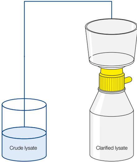
Figure 2 NucleoBond® RS Bottle Top Filter Type 2 setup
